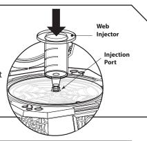
4. Once the gel has liquified, remove the gel packet from the beaker. With assistance from an adult, carefully trim the gel packet with scissors along the dotted line and squeeze the gel into the Web Creator Lab Injector.
