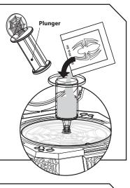
5. Insert the plunger into the Web Injector and gradually press down to inject gel into the Web Plate until the web cavity is full.
