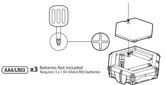
**14** Put the cover onto the top of the chamber. Slide the switch to turn on the light.
